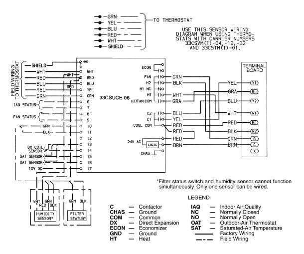
Fig. 9 — Apollo Control Wiring Schematic — 50HJQ, 12<sup>1</sup>/<sub>2</sub> and 15 Ton Units
